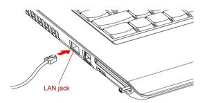
Figure 4-19 Connecting the LAN cable
